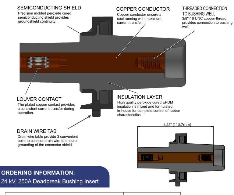
250A, 24 kV Deadbreak Bushing Insert
