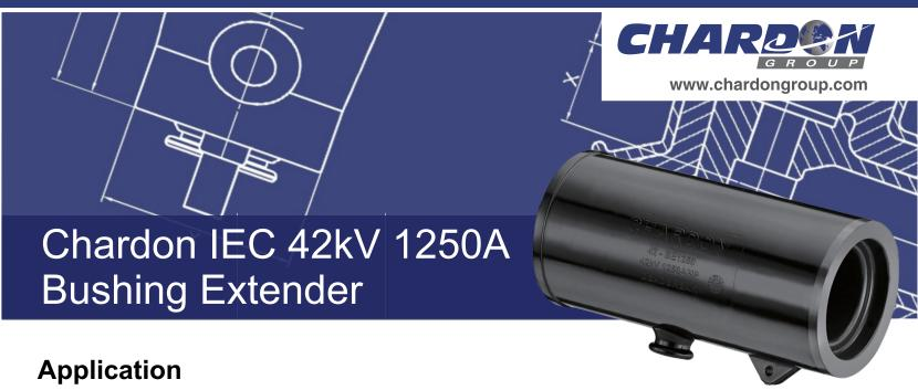
The Chardon 42kV 1250A bushing extender can be used for temporary or permanent applications and provides a submersible, fully shielded insulated connection between energized bushings and Chardon 42kV rear Tbody product(42-RDT1250).
