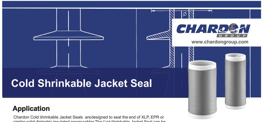
Chardon Cold Shrinkable Jacket Seals are designed to seal the end of XLP, EPR or similar solid dielectric insulated power cables The Cold Shrinkable Jacket Seal can be used when installing elbows or other cable accessories. The product is submersible and UV resistant. The spiral tube design allows the users to remove the inner tube easily during installation. The rubber tube provides sealing and protection on jacketed concentric neural cable. No additional tools are required for installation.
